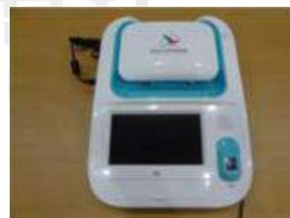
**Figure 3 Identification Machine (checks the voters ID, enter signature or fingerprint)**
